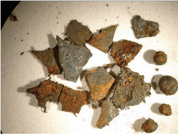
Figure 24. Hammerscale and spherical iron droplets, byproducts of blacksmithing
