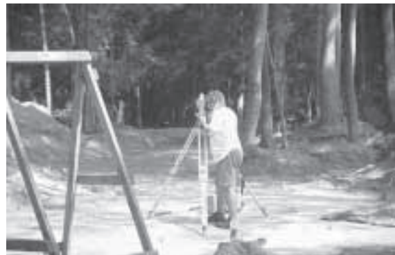
Figure 2. Mapping the site's features with the total station laser transit.
